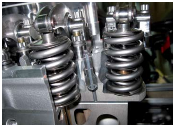
Cutaway of the 2009 Toyota Cup engine showing valve spring cooling oil spray jets (photo: Martin D Clark)
